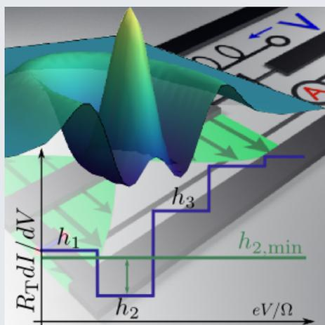
Differential conductance  $dI/dV$  versus dc bias voltage  $V$  for a tunnel junction coupled to a microwave cavity initially prepared in the Fock state  $n=2$ . The striking signature of a non-classical state here is the strongly non-monotonic dependence of the first few conductance plateaus on voltage; in particular, the height of the second plateau ( $h_2$ ) is smaller than the first ( $h_1$ ). This is in one to one correspondence in the Fock state with exactly two photons in the cavity
