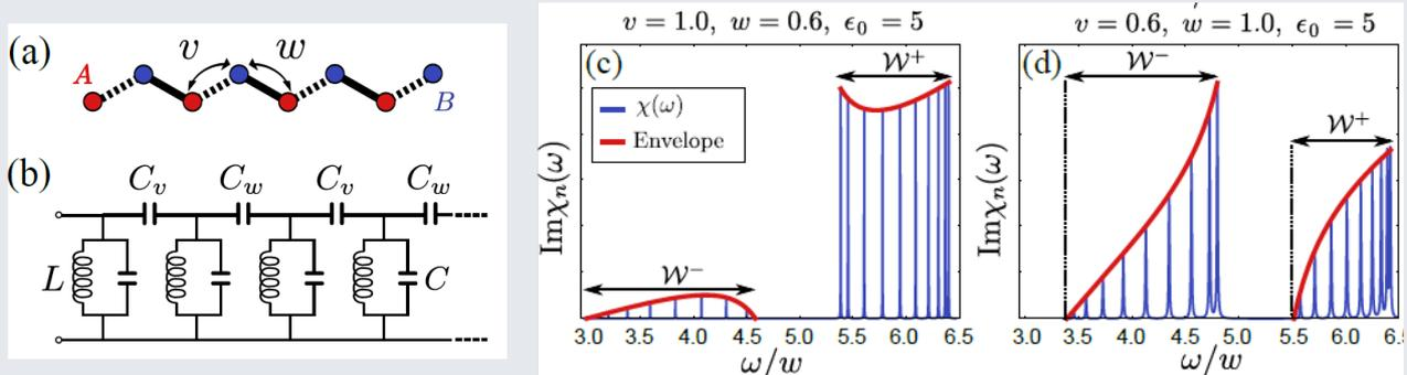
We show the emergence of topological Bogoliubov bosonic excitations in the relatively strong coupling limit of an LC (inductance-capacitance) one-dimensional quantum circuit (see figures (a-b)).
