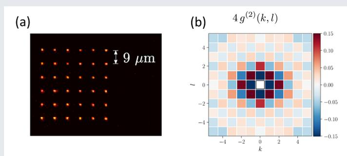
**Quantum simulation of an Ising antiferromagnet using individual Rydberg atoms.** (a): fluorescence image of single atoms, arranged in a  $6 \times 6$  square array. (b): spin-spin correlation function of the system after a quasi-adiabatic sweep of the system parameters, showing the onset of antiferromagnetic order, albeit with a finite correlation length.
