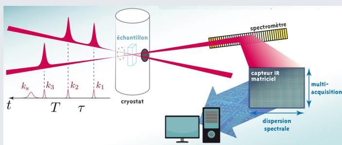
2D-IR scheme based on a pump-probe geometry with nonlinear signal dispersed onto a grating
