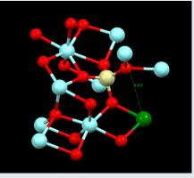
Reduced crystalline cell of yttrium orthosilicate with erbium dopant in green. Yttrium ions are in blue, oxygen in red and silicon in yellow form the Y2SiO5 matrix. Despite the large number of yttrium close to erbium, we have shown that a specific Er-Y pair can be optically addressed (here separated by 5.4A represented by a dashed green line)
