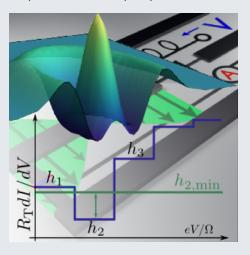
Differential conductance dl/dV versus dc bias voltage V for a tunnel junction coupled to a microwave cavity initially prepared in the Fock state n=2. The striking signature of a non-classical state here is the strongly non-monotonic dependence of the first few conductance plateaus on voltage; in particular, the height of the second plateau (h2) is smaller than the first (h1). This is in one to one correspondence in the Fock state with exactly two photons in the cavity
