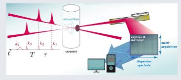
2D-IR scheme based on a pump-probe geometry with nonlinear signal dispersed onto a grating
