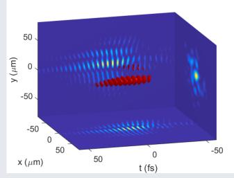
3D reconstruction of the E-field amplitude of the UHI 100 laser, measured at the focal point, by INSIGHT technique. On each side, the field projection on each coordinate is reported.
