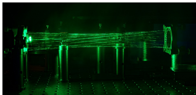
Figure 8. A green laser beam propagates in a multipass cell used for nonlinear temporal compression down to the few cycle regime (project CellComp)
